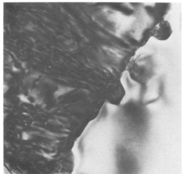
Figure 7 The edge of a cBN grain, with [1\ 1\ 0] approximately parallel to the beam. Field width 0.8\ \mu\text{m} . The AlN rind runs diagonally across the field from lower left to top right and is about 20 nm thick except for nodules about 60 nm thick. A defect-free region of the AlB 2 network, appearing light on the print, occupies the lower right-hand part of the field.
