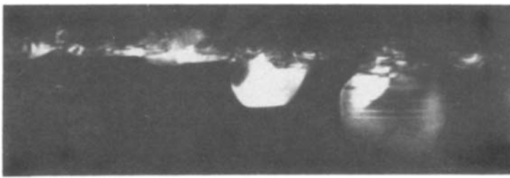
Figure 9 Dark-field image formed with an AlN reflection showing central part of the AlN rind along the grain edge in Fig. 7a. Field width 0.6\ \mu\text{m} , printed rotated 55^\circ clockwise with respect to Fig. 7; the AlN [0001] direction is now vertical. Contrast in the AlN is highly uneven.
