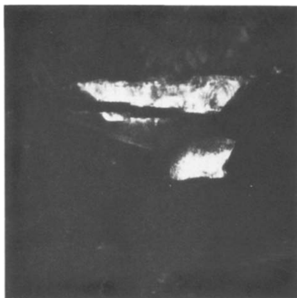
Figure 16 Dark-field image from the same area as Fig. 13, formed using an \text{AlB}_2 reflection. The \text{AlB}_2 that has remained attached to the upper grain is in strong contrast while the rest has become slightly misoriented and does not show such strong contrast. It can be presumed that most of the \text{AlB}_2 in the cavity between the three cBN grains had the orientation illustrated in Fig. 14 before the specimen was thinned.
