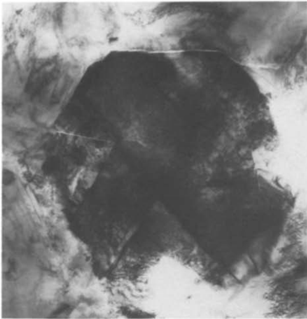
Figure 2 A bright-field TEM section through a cBN grain. Field width 6\ \mu\text{m} . The grain has [1\ 1\ 0] parallel to the beam and [00\ 1] is approximately vertical on the print. White areas on the print correspond to the specimen having thinned right through. Image recorded at 300 kV.
