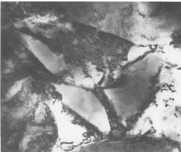
Figure 18 A region occupied by fragments of cBN derived from the same original grain. Field width 4.5 μm. The fragments show varying degrees of plastic deformation. Image recorded at 300 kV. The location of the three weakly diffracting cBN fragments referred to in the text are, with respect to the field centre, lower right, below and upper left. The completely white area towards the bottom of the field is a hole in the specimen.
