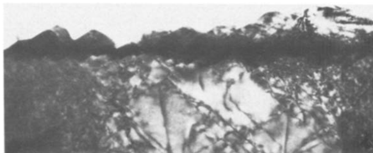
Figure 12 A cBN edge that does not represent a cube or octahedral facet. Field width 1.4 \mu\text{m} . The beam direction is parallel to [110] and [001] is horizontal on the print. Individual crystallites of the \text{AlN} rind exhibit well-developed (0001) faces. Image recorded at 300 kV.
